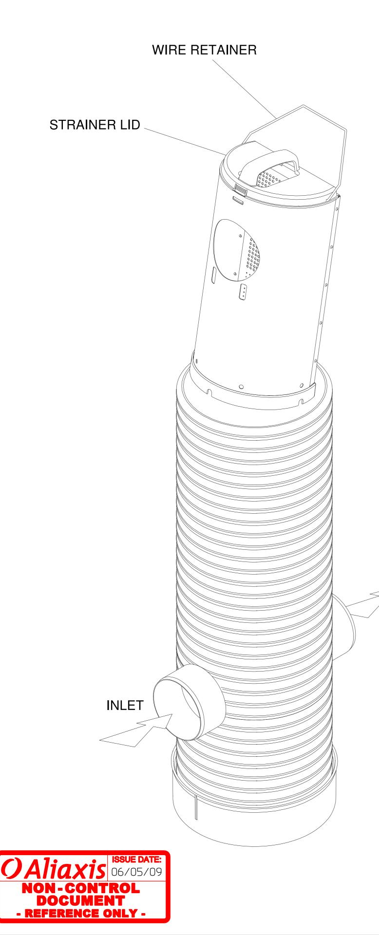
NOTE: WHEN FITTING UG61 STRAINER, THE LEAF GUARD SHOULD BE REMOVED FROM THE UG60 SILT TRAP AND DISCARDED
