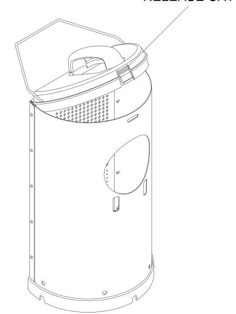
REF: SILT TRAP INST. MC6167 ISS.2 MAY 2009 TO EMPTY STRAINER, PRESS RELEASE CATCH & REMOVE LID. WHEN REPLACING LID MAKE SURE HINGE LEDGE IS LOCATED BENEATH FACE PLATE FLANGE BEFORE REPLACING STRAINER REMOVE ANY SILT FROM BASE OF SILT TRAP
